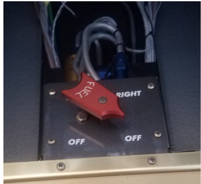
The Fuel Shutoff Installed
