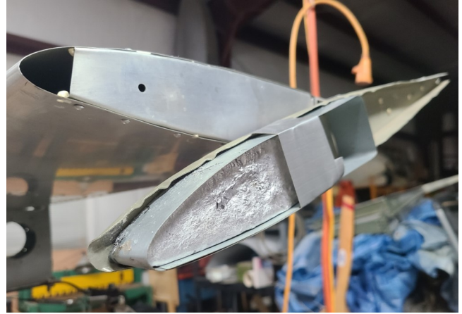
Elevator Ballast weights taped in place
