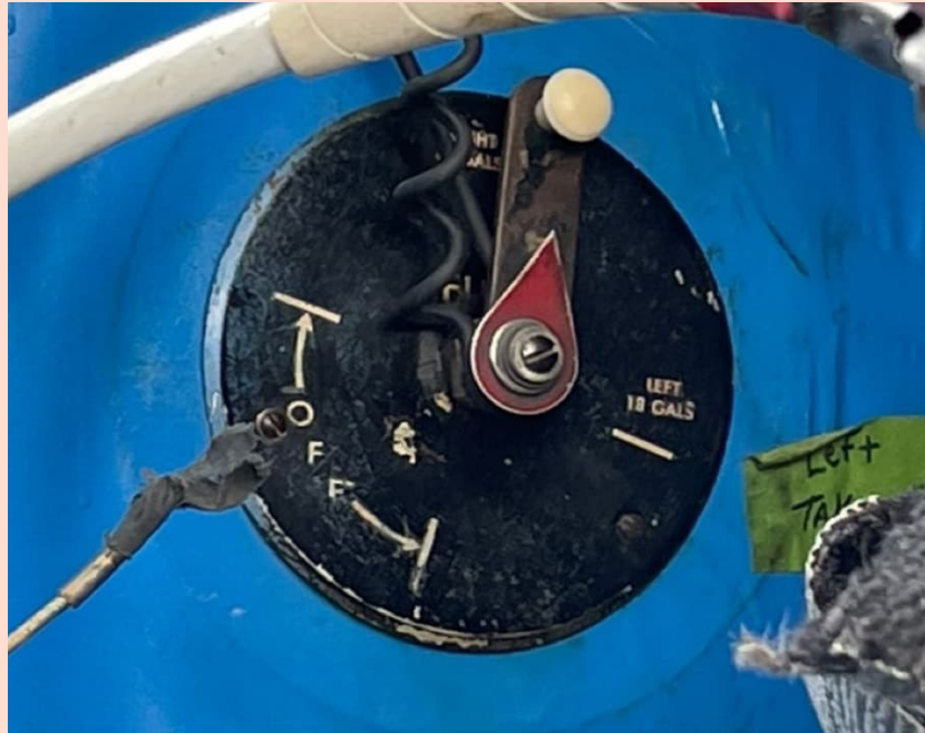
The fuel selector in the Tri-Pacer. (All Photos from the NTSB docket)
